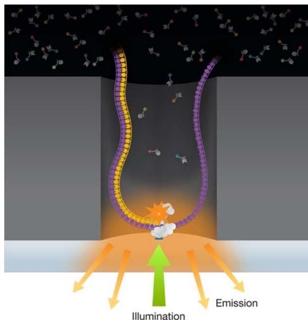
**Fig. 8** Single nanometric aperture for real-time single-molecule DNA sequencing. A DNA polymerase molecule attached to the bottom surface is used to successively incorporate fluorescent nucleotides complementary to the DNA strand, causing fluorescence bursts for each incorporation process (see text for details). Image copyright of Pacific Biosciences Inc., reprinted with permission
