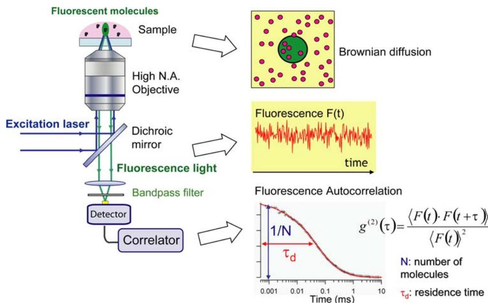
number fluctuations, it is particularly efficient for small  $N$ , typically ranging from 0.1 to 100 molecules, which corresponds to concentrations from 0.4 to 400 nM in a standard confocal volume ( $0.5 \text{ fL} = 0.5 \times 10^{-15} \text{ L} = 0.5 \mu\text{m}^3$ ).
