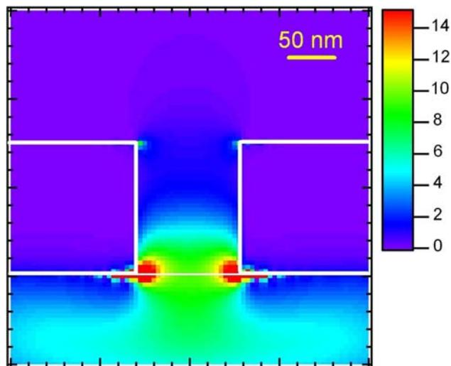
**Fig. 7** Three-dimensional finite-element time-domain simulation of the intensity distribution (*linear scale*) for a nanoaperture milled in gold with 120-nm diameter and 150-nm thickness. The substrate was taken to glass, while the upper medium and the aperture inside were taken to pure water. The illumination was set to uniform intensity distribution (*plane wave*) with free space wavelength of 633 nm, and linear polarization parallel to the plane viewed here
