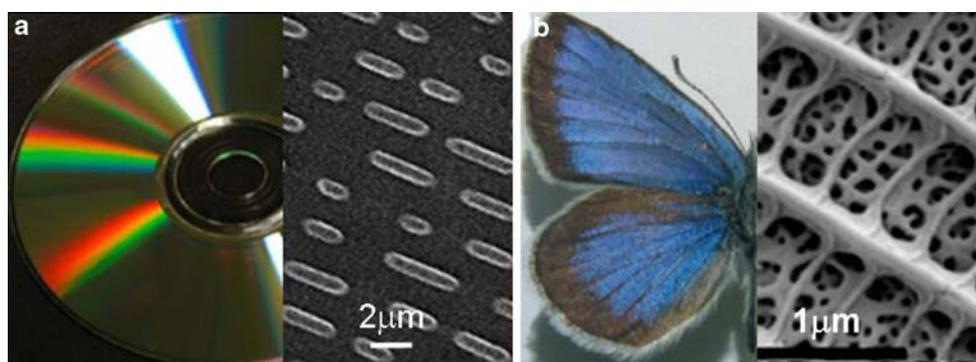
**Fig. 1** Diffraction of light with nanophotonic structure. **a** A compact disc and a closer look of its surface. **b** Male butterfly *Albulina metallica* and a closer look of its dorsal wings (from (Biró et al. 2007))
